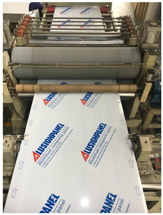
The last step : collecting the aluminum composite panel and packing . (Our factory also have update the Automatic machine doing this ) .
