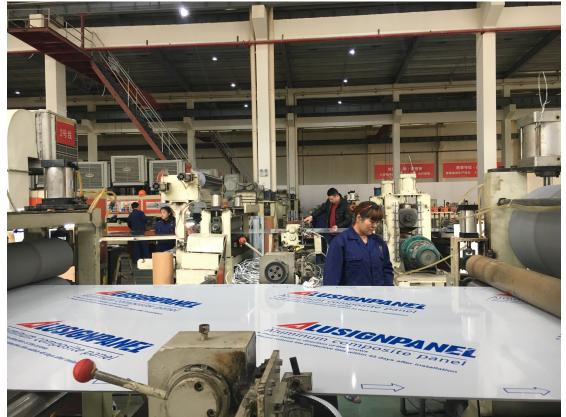
The six step : Aluminum Composite Panel levelling before length cut . ( so the panel custom length are easy for our Alusignpanel factory , recommend between 2.0 meter and 5.8 meters basic on the containers loading ) .
